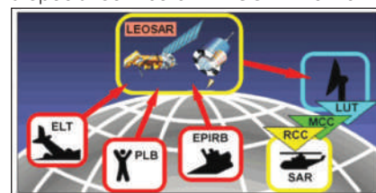
▲ Fig. 4 LEOSAR Cospas-Sarsat system concept. Source: Cospas-Sarsat.
